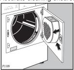
If necessary the filters can be cleaned under running water using a brush. In this case remove the filter in the door opening as per picture (it can be positioned with the tooth facing to the left or to the right).
